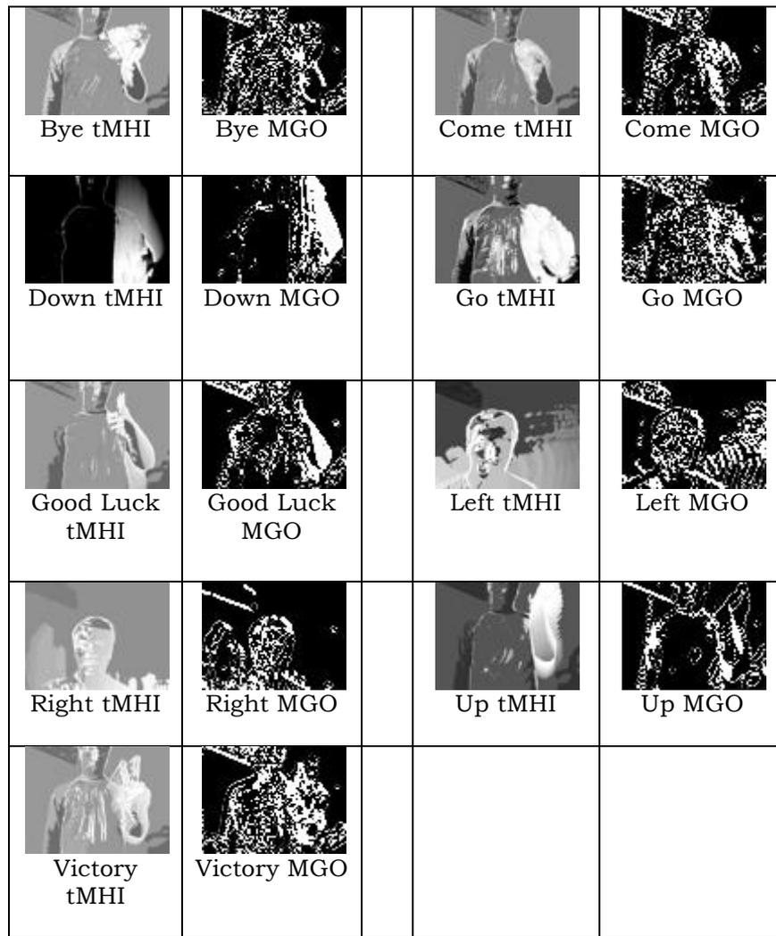
**Figure 4.1:** Example tMHI and MGO for the 9 gestures used in experiments.
