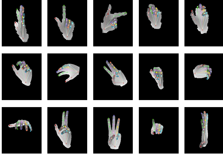
Fig. 5. Examples of hand pose estimation. The top row is Kinect depth images and bottom two rows are artificial data.
